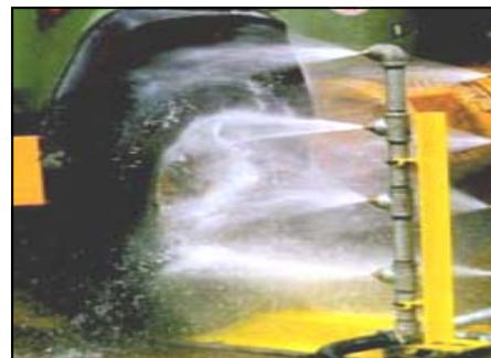
A high pressure spray tire wash cleaning system (Mark Kestner).
