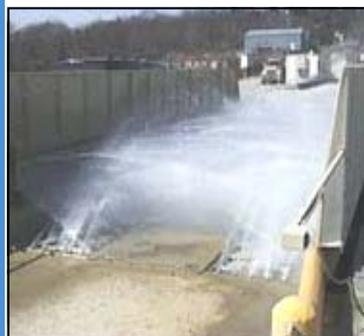
A low pressure tire wash cleaning system (Mark Kestner).
